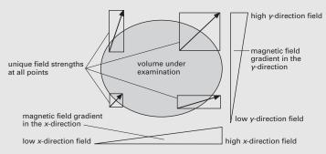
MRI. The way unique field strengths are produced at different points in a specimen
