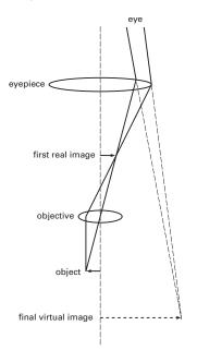
Microscope. Compound microscope.
