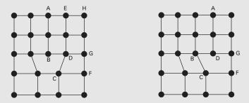
**Dislocation in a two-dimensional crystal.** The extra plane of atoms AB causes strain at bond CD. On breaking, the bond flips across to form CB. This incremental movement shifts the dislocation across so that the overall effect is to slide the two planes BDG and CF over each other.
