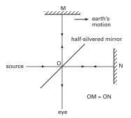
Michelson-Morley experiment. Michelson interferometer. tion, or orbital motion, is not identical to its speed at right angles to this direction. No shift was observed. An explanation was finally provided by the \*Lorentz–Fitzgerald contraction, which provided an important step in the formulation of Einstein's special theory of \*relativity and the abandonment of the ether concept.
