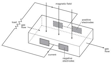
Magnetohydrodynamics. Magnetohydrodynamic generator.
