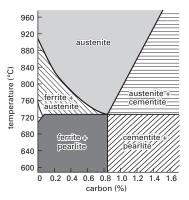
Steel. Phase diagram for steel.
