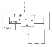
Solar cell. A silicon p-n junction.
