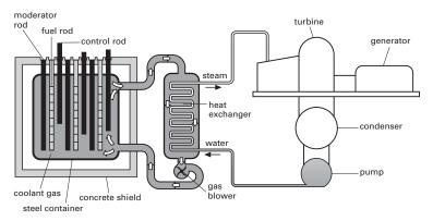
Nuclear reactor. A schematic diagram of a gas-cooled reactor.
