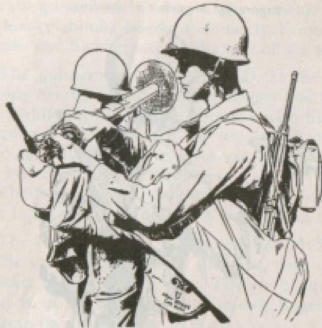
Ⓢ Raises tail latch; pushes rocket completely into launcher.
