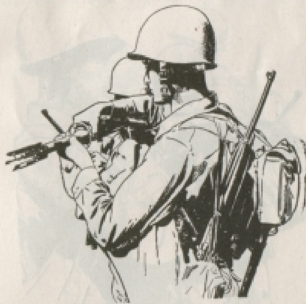
ⓑ Inserts body of rocket partially into launcher; removes safety pin.
