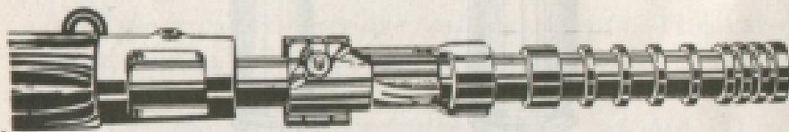
Figure 19. Launcher M1 attached to muzzle of rifle by clamp and wing nut.
