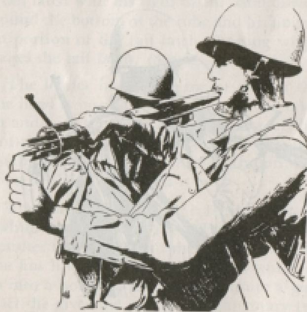
Ⓢ Removes contact wire from rocket fin.
